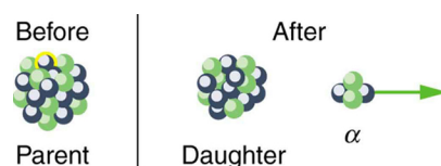
Figure 31.17 Alpha decay is the separation of a {}^4\text{He} nucleus from the parent. The daughter nucleus has two fewer protons and two fewer neutrons than the parent. Alpha decay occurs spontaneously only if the daughter and {}^4\text{He} nucleus have less total mass than the parent.
